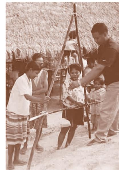
**Photo 2** The A-frame used to locate contour lines
