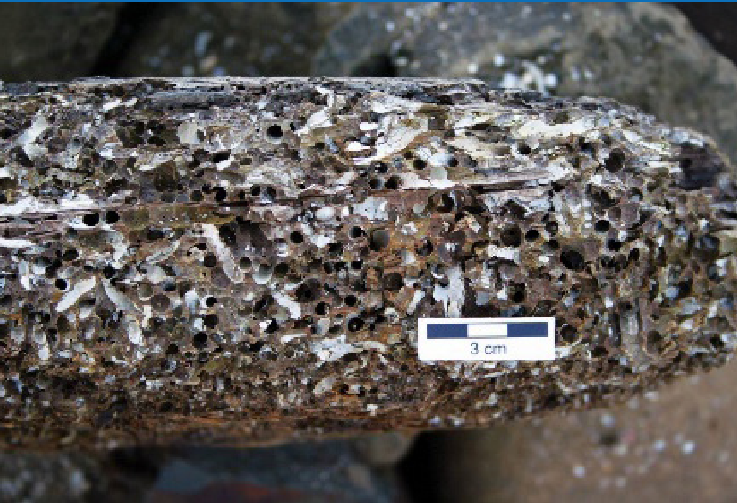
• Fig. 20: Ship timber damaged by ship worms. © Michael C. Rygel via Wikimedia Commons
