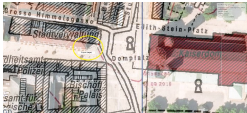
Figure 8. Sample image using the corner of a building as a control point. The control point selected on the raster was first clicked, followed by the same point on the basemap.
