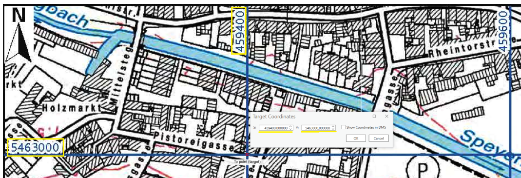
Figure 3. Captured image after inserting the coordinates (highlighted in yellow) of the intersections of the cartesian axes of the grid into the georeferencing tool.
