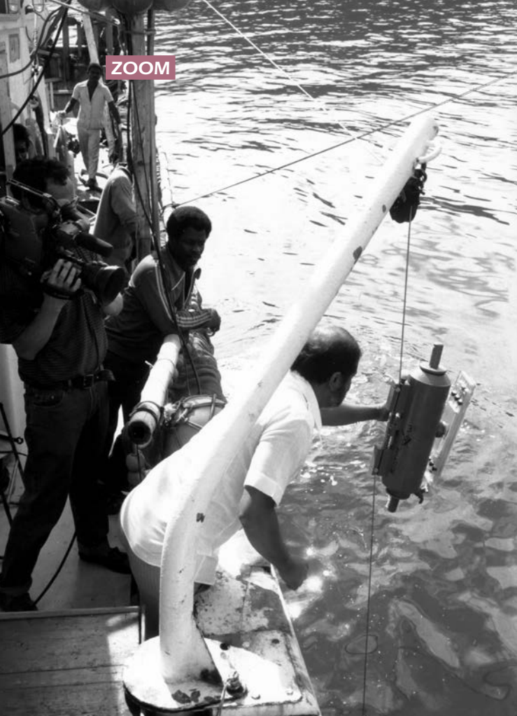
Samples of sea water being taken to measure temperature and salinity by the National Centre of Oceanographic Research, at Nosy Bé, Madagascar, 1989. The project was part of UNESCO's Intergovernmental Oceanographic Commission (IOC).
