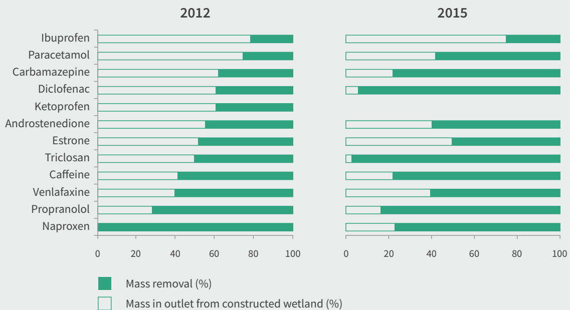
Figure | Removal rates for different pharmaceuticals in a pilot-scale constructed wetland in different operating conditions in 2012 and 2015
