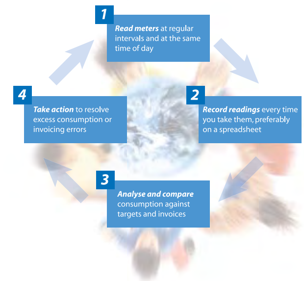
Figure 1 Reading meters for energy management
